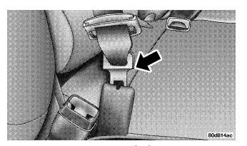
**Inserting Latch Plate**
